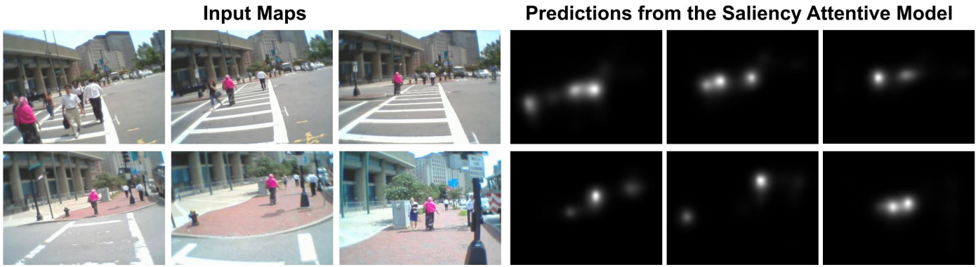
Fig. 19. Examples of Saliency maps predicted on the SERI Homonymous Hemanopia Dataset using a modified Attentive ConvLSTM with learned priors
